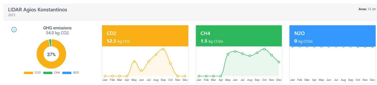
Figure 6. CMM dashboard interactive chart for detailed GHG emissions per area (LiDAR device)
