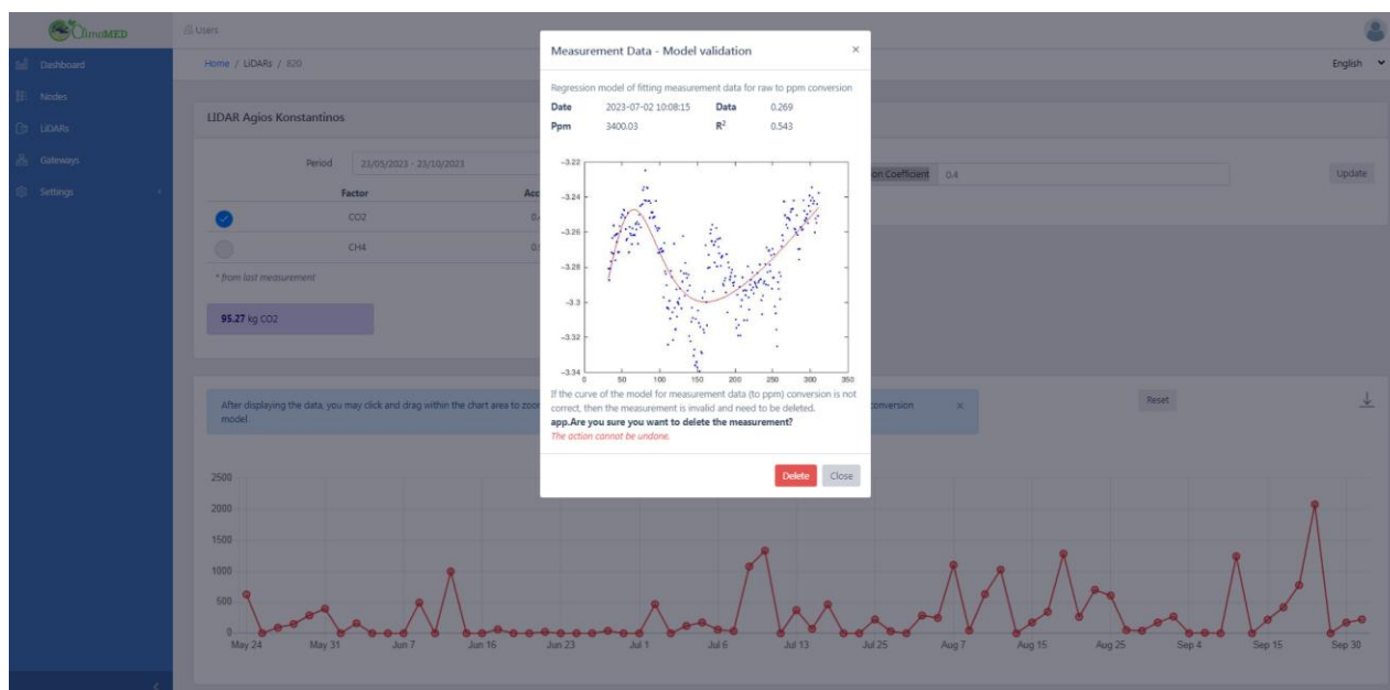
Figure 14. Modal window displaying LiDAR data model information to be cross-validated by experts
