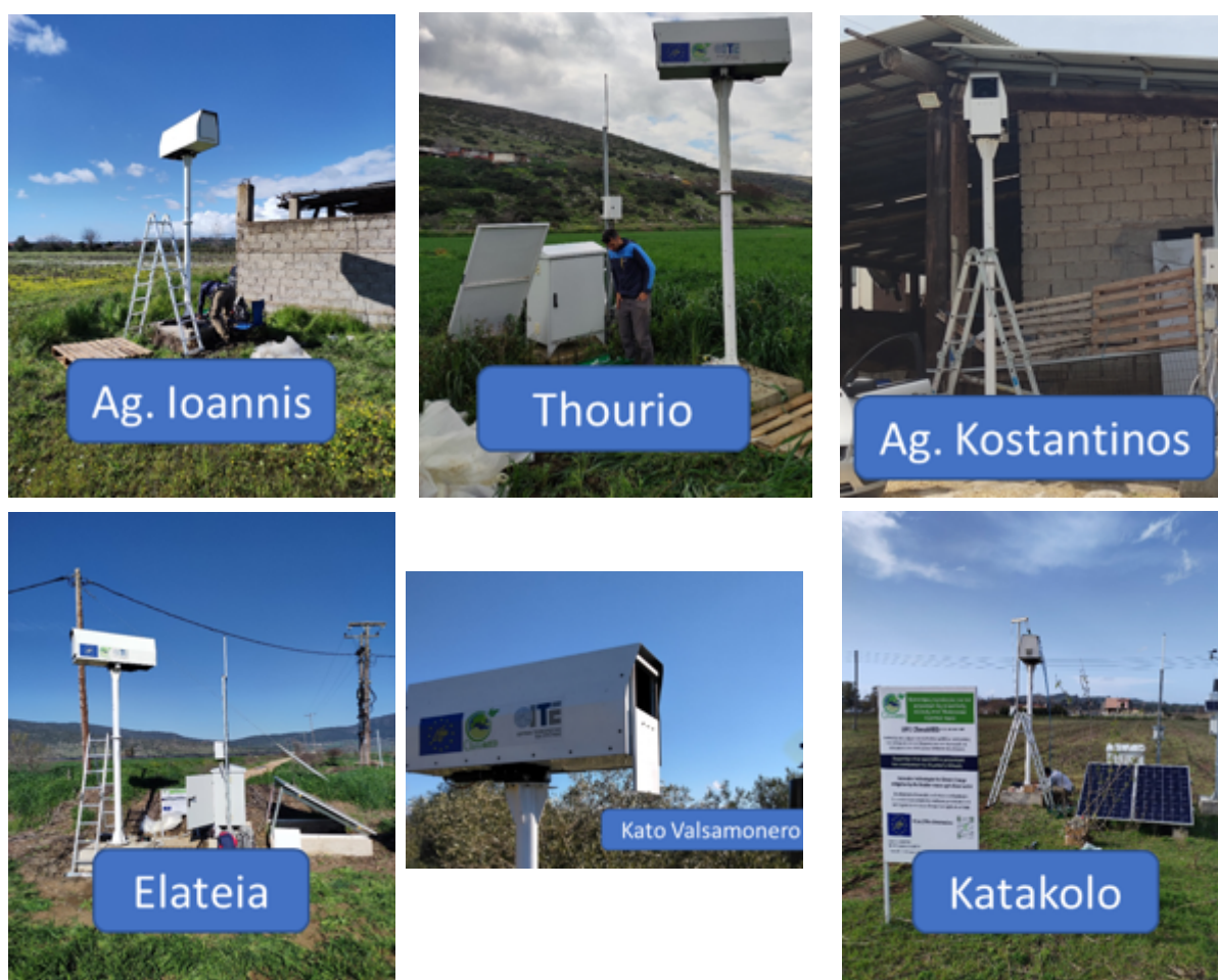
Figure 3: the six LIDAR Devices in Greece continued to monitor the greenhouse gases until the end of the project
