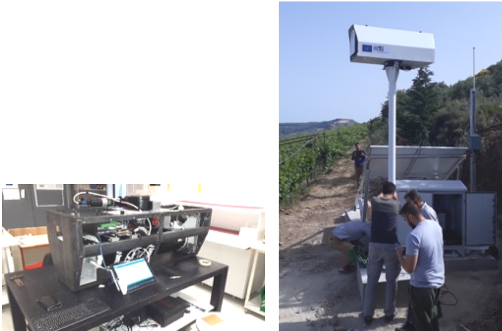
Figure 1. The LIFE Climamed greenhouse gas measurement system, consisting of the LIDAR measurement device, meteorological station, and solar panel.
