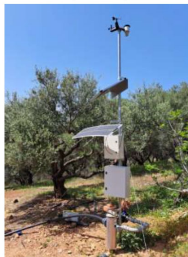
Figure 6 Smart electrovalves and M/S and datalogger of IWAM system
